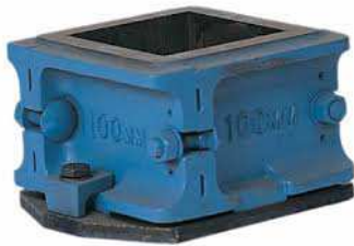
Figure 2.4: Cube Mold (100mm x 100mm x 100mm)
