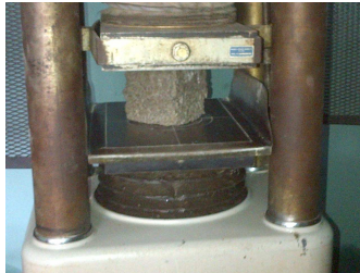
Figure 2.1: Crushing Machine manufactured by Engineering Laboratory Equipment Limited (ELE)
